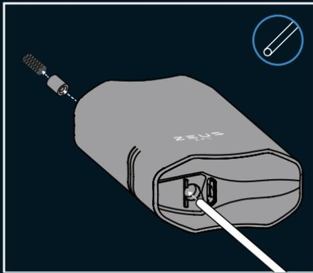
Insert the **Flow Sink Tool** from the bottom of the air path and carefully push to remove the **Flow Sink** or the ZEUS ARCPD™. Once cleaned, reassemble fully [**Flow Sink & Flow Sink Screen**] through the top of the **Heating Chamber**.
