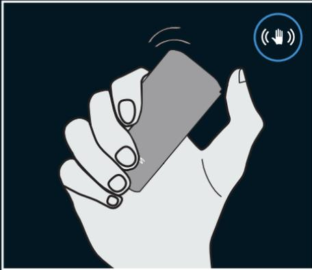
To check battery level during operation, shake the device twice during use. The **LED Status Interface** will display the level in red.
