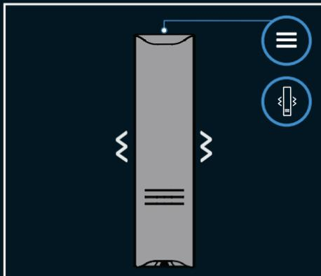
Hold the **Power Button** for 2 seconds to turn the device on/off. A long vibration indicates that the device is turned on/off.
