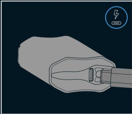
Plug the provided **USB-C Cable** into a USB charge adapter with the rating not higher than  $5\text{ V} = 2.5\text{ A}$  and connect to the **USB-C Port**. When the ZEUS ARC™ has finished charging, all LED lights will be solid red.
