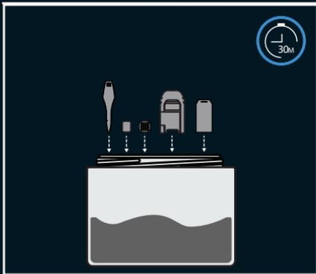
Remove the **Multi-Tool**, **Flow Sink**, **Screen**, **Mouthpiece GTS** and **Heat Sink GTS**. Place displayed parts in a mixture of ZEUS PURIFY™ or alcohol for a maximum of 30 minutes [exception **Mouthpiece GTS**]. Subsequently, rinse all parts with water. The **Heat Sink Cover GTS** should be removed from the **Heat Sink GTS** prior to rinsing.
