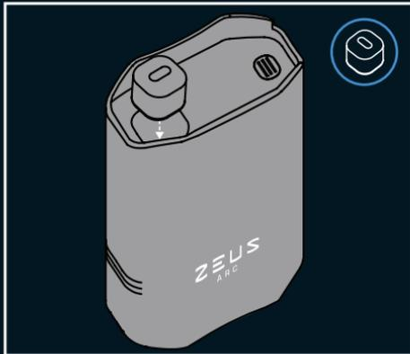
To use less botanical, place the **Spacer** at the bottom of the **Heating Chamber**.
